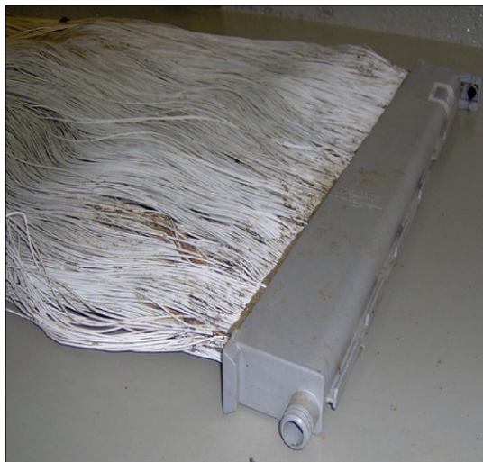
Fig. 13. Membrane technology membrane module element in Karcag [3]
