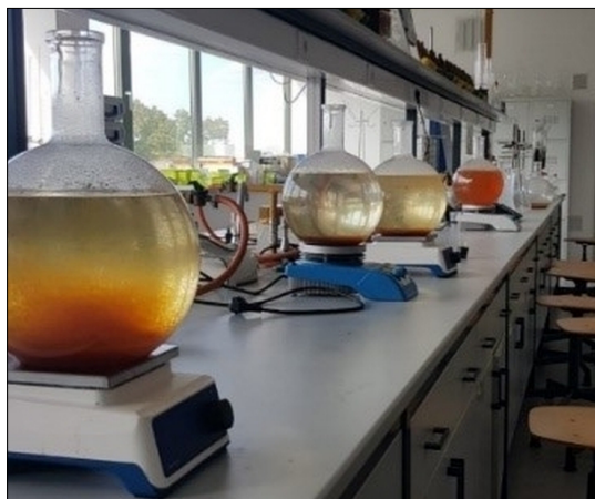
Fig. 1. Coagulation-flocculation chemical treatment.
