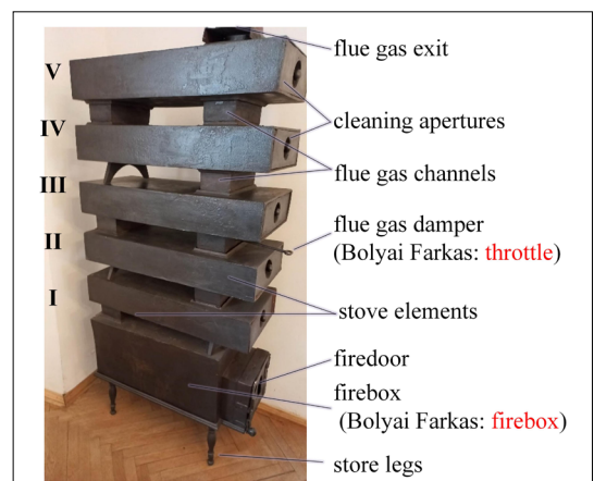
Fig. 1. The construction of the studied Bolyai stove.
