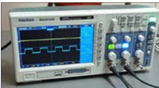
Figure 9. Waveforms sent to motor controllers.
