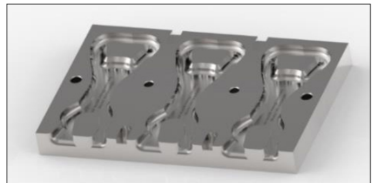
Figure 2. The casting tool model.
