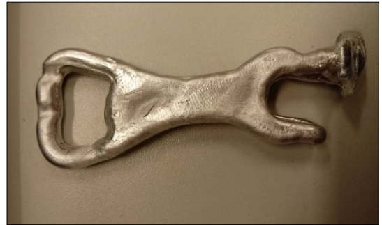
Figure 8. Absorption and hot cracking.
