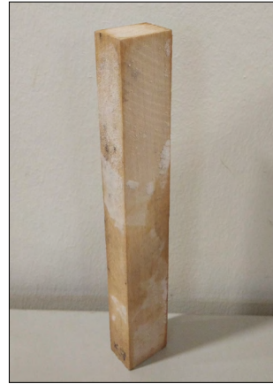
Figure 7. 20×30×200 mm beech specimen.
