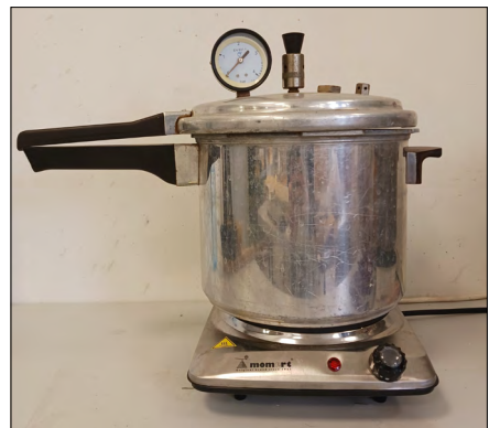
Figure 4. The vessel used for steaming the specimens.
