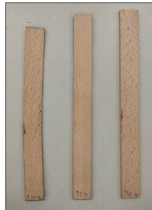
Figure 8. Thin specimens cut from larger beech specimens in order of compressed and fixated for a long time, fixated for a short time and untreated.
