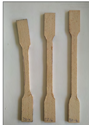
Figure 9. Fixated for a long time, fixated for a short time and untreated small samples in sequence, with a profile designed for tensile testing.
