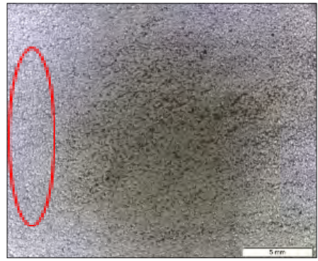
Figure 10. Scratched (left) and wire-brushed 2304 specimens after two weeks, scale is 5 mm.
